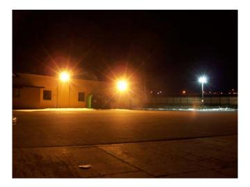
Please consider replacing (or retrofitting) these 3 lights with full cutoff fixtures that direct the light downwards and across the parking lot, where the light is needed for public safety.
