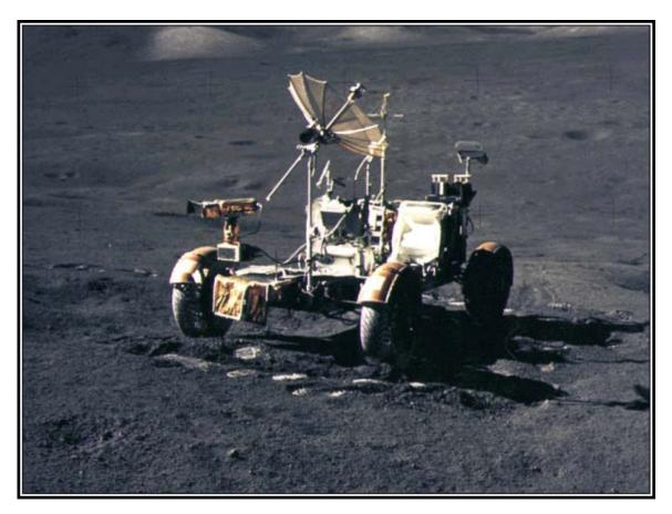
An average speed of 9.6 km/hr was achieved, and speeds up to 12 km/hr were attained over level lunar terrain. The total distance traveled, was 27.9 km, corresponding to a map distance of approximately 25.3 km.
