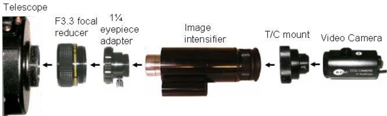
Figure G-6. Video Camera, image intensifier, f3.3 focal reducer attached to telescope.
