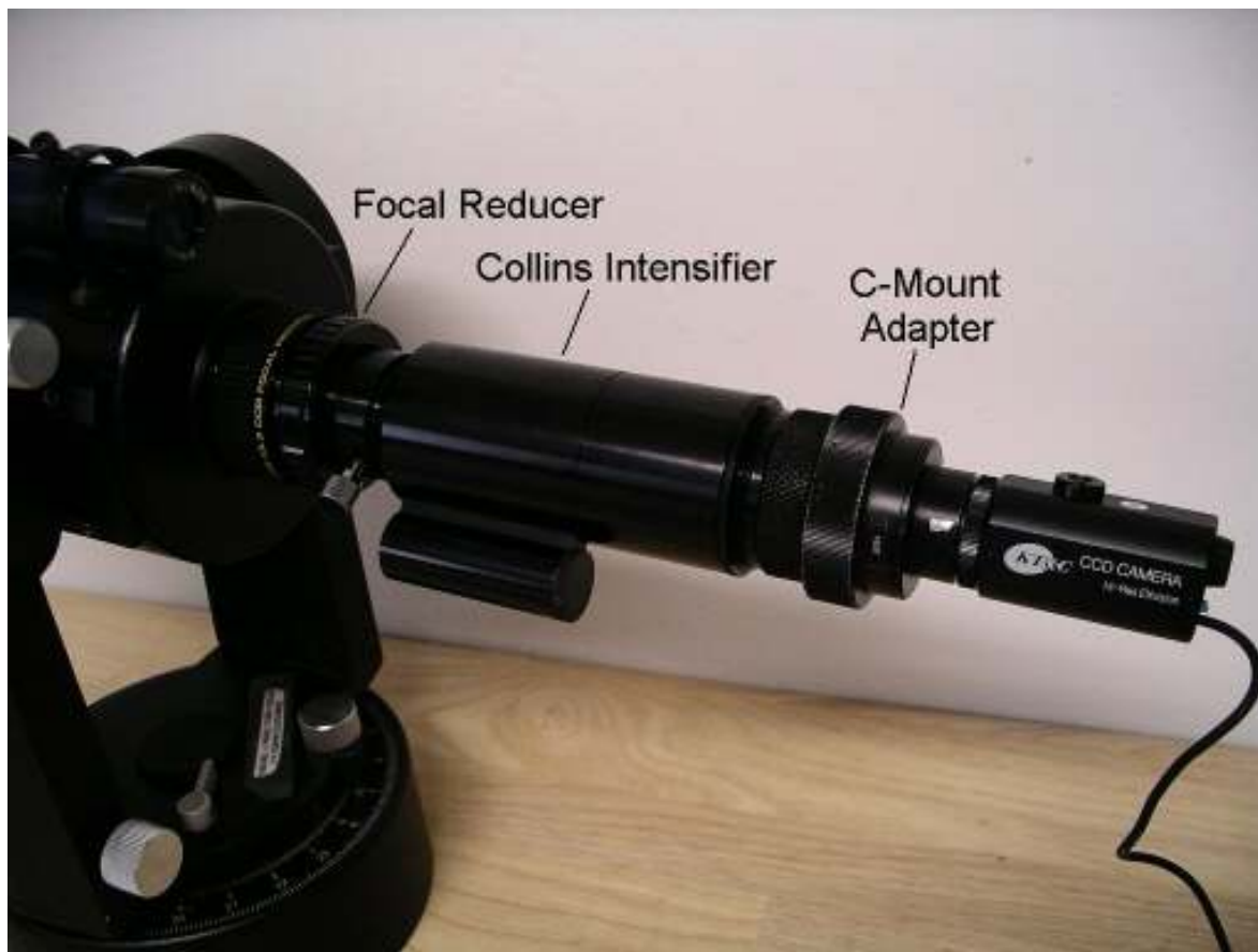
Figure 6.9. PC-164C camera attached to Collins I 3 Image intensifier. The Collins I 3 piece is attached to a f3.3 focal reducer at the back of the telescope. The Collins I 3 is powered by a 3V lithium battery with its holder attached to the bottom of the Collins tube.
