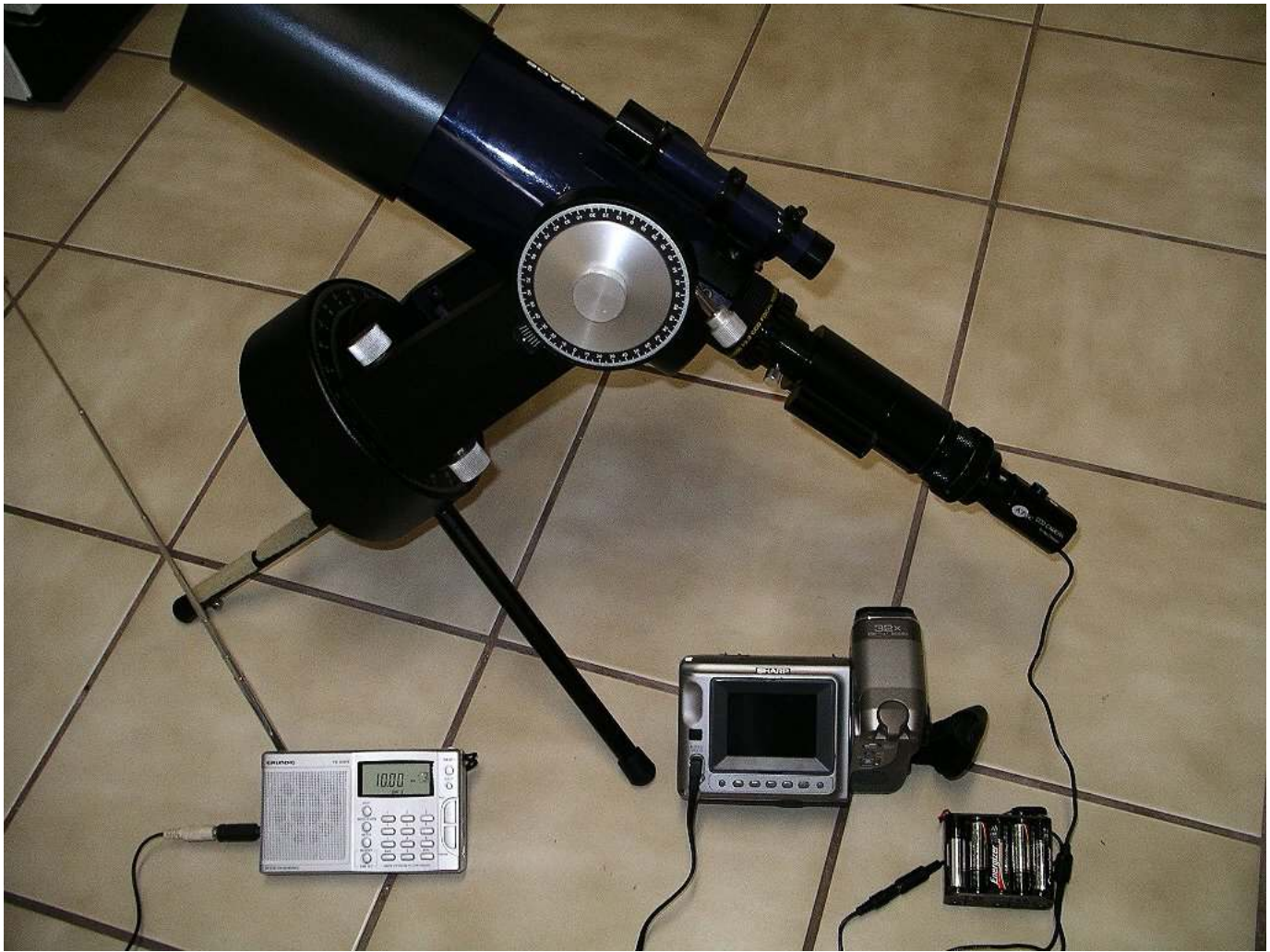
Figure 8.6. Portable video occultation system. The PC-164C camera and Collins I 3 intensifier are attached to the f3.3 focal reducer on the back of a 4 inch telescope with dew shield. The camcorder receives audio input from the shortwave radio and video input from the PC-164C camera. The AA battery pack (lower right) powers the PC-164C camera. This system can video record stars to m_v = 12.0 in a dark sky and the whole system fits in a medium size backpack or large briefcase fitting in the overhead compartment of airplanes.
