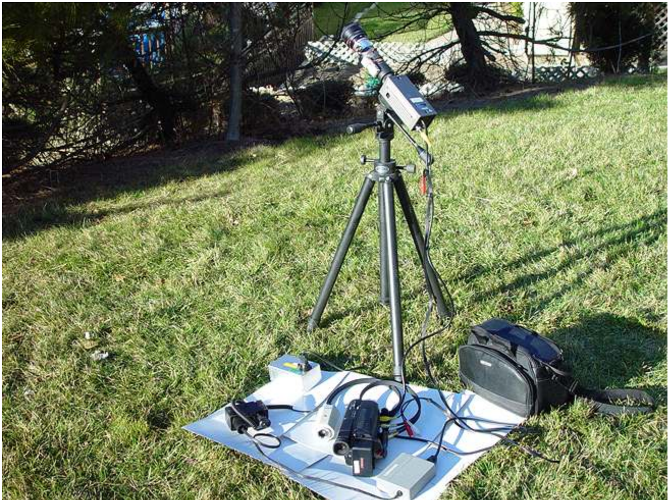
Figure 10.1 Remote video station. Equipment consists of a video camera attached to a stationary tripod, a shortwave radio, power source, and a camcorder to record the event. Courtesy David Dunham.
