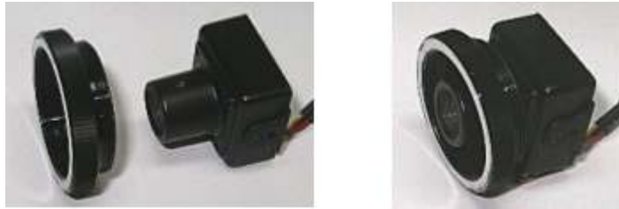
Figure D-1. Use of a C-ring for attachment (glued) to Supercircuits PC 180XS camera.
