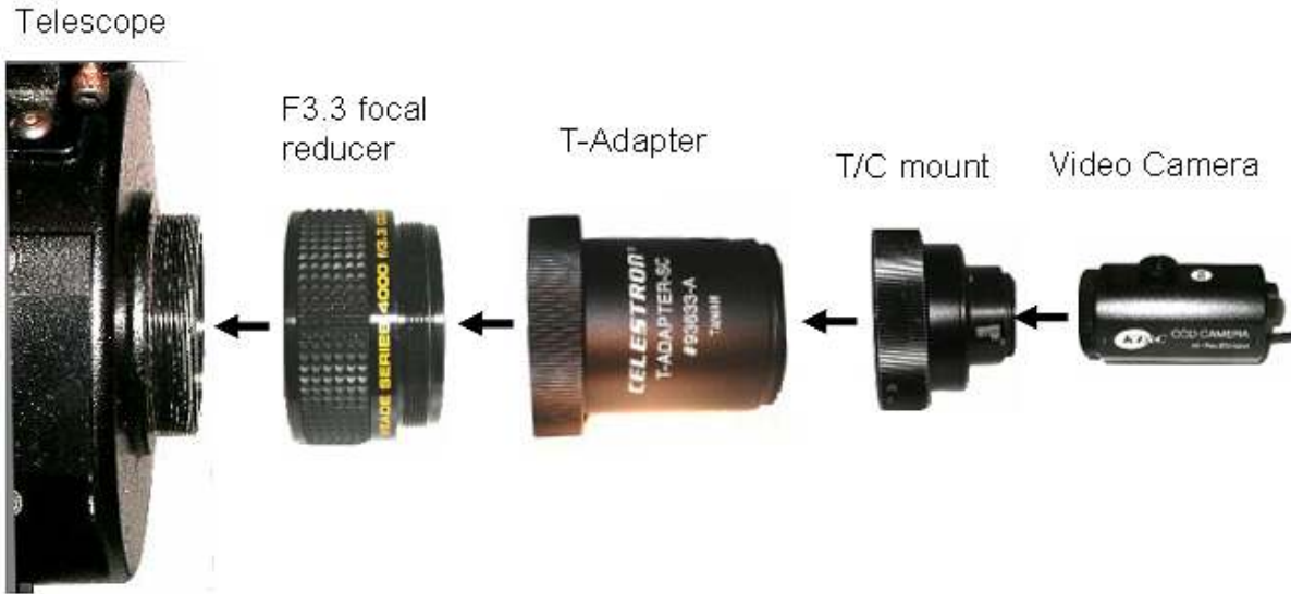
Figure G-4. Video camera adapted to telescope with f.3 focal reducer and T-adapter.
