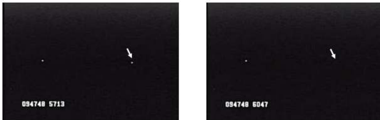
Figure 8.10. Successive GPS time inserted video frame from the occultation by the asteroid 372 Palma on 26 January 2007. Note the disappearance of the target star in the right video frame. The displayed time for the left frame reads 9h 47m 48.5713 sec and for the right frame 9h 47m 48.6047 sec UT (0.033 sec difference). This video was made using a Supercircuits PC-164 camera. The target star is at the right of each frame and a field star is at the left of each video frame. Field size is 15 x 20 arc minutes. From video by Richard Nugent.
