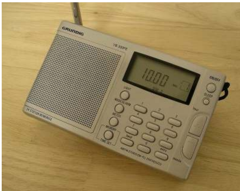
Figure 3.3 Digital Tuning shortwave radio set to WWV 10 MHz. Radio is Grundig model YB 300PE and is a compact 5.5" x 3.5" x 1".
