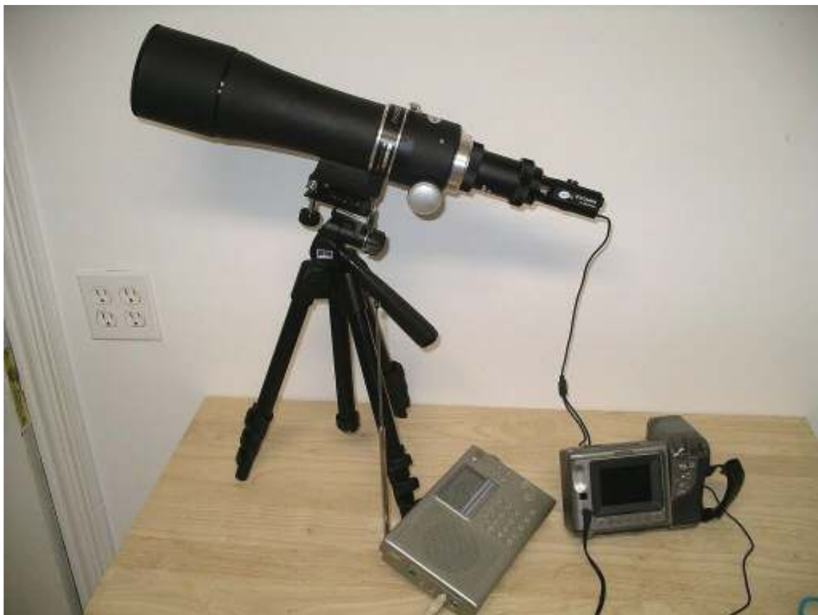
Figure G-7. Unattended video station setup.
