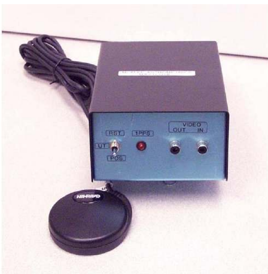
Figure 8.11. McAfee Astrometrics GPS Video Time Inserter. The toggle switch at left has 3 positions, RST (reset), UT (Universal Time) and POS (position). In the POS mode the unit displays latitude, longitude and date information to the output video monitor, camcorder or VCR. In UT position, the toggle switch outputs UT to 0.001 sec. The RST is a reset function used at the start of a recording session. The 1PPS LED light blinks once per second when the unit has a fix on the GPS satellites (this could take up to several minutes) letting the user know the unit is working. The VIDEO OUT IN are jacks for input of cables to a video camera and output to a camcorder or VCR. The hockey puck looking object in front of the VTI unit is the Garmin model G18LVS GPS receiver that outputs the 1 pps signal to the VTI unit along with UT and position information. It plugs into the back of the unit and has a magnetic base for easy attachment to metal (such as a car roof) up to the length of the cord.
