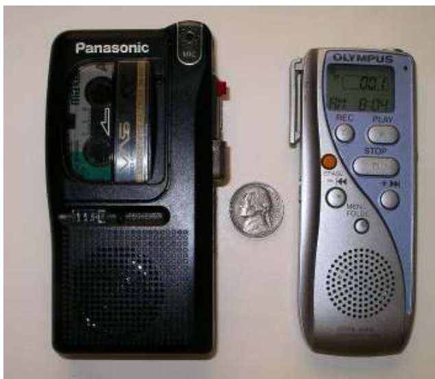
Figure 8.1. Micro-cassette recorder (left) and digital voice recorder (right). Digital voice recorders are not affected significantly by temperature variations and have no moving parts.
