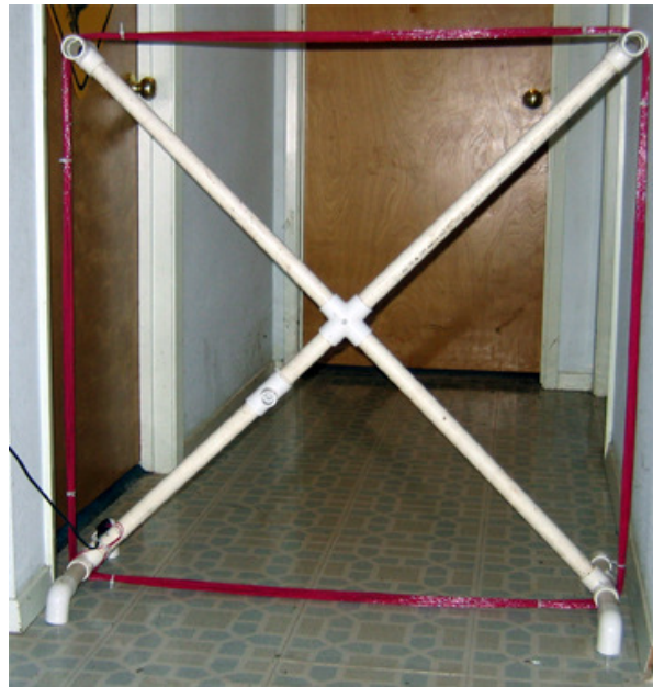
Note the use of zip ties to make sure the wire windings stay together.
