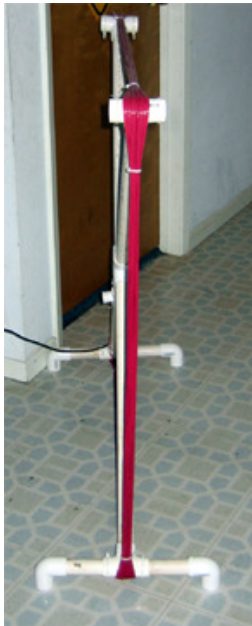
Note the use of zip ties to make sure the wire windings stay together.
