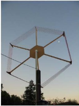
A loop antenna to pick up VLF signals reflected from the ionosphere
