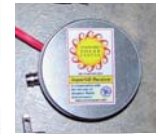
A PreAmp to raise very small signals to a level can be captured by a PC sound card.
